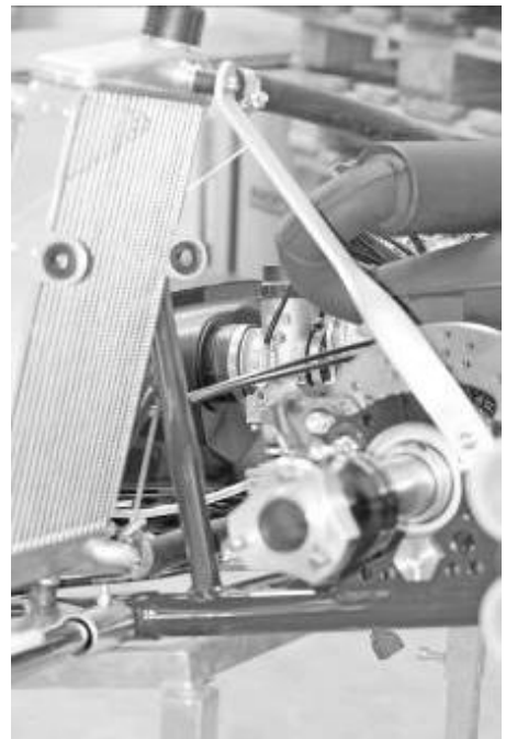
Foto of the frame from the side with the section of the supports for the radiator (radiator mounted)
