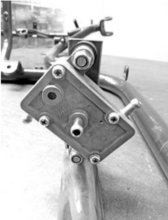
Foto of the frame with the section of the support for the fuel pump (fuel pump mounted)
