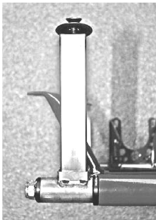
Foto from the steering column with the section with the knurling for the steering wheel hub (knurling according to DIN 82 - RAA1).
